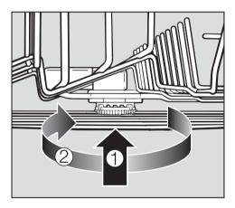
■ Lift up the **middle** spray arm, ①, to engage the ratchet and unscrew the spray arm, ②.
